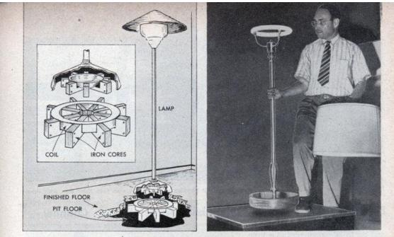
Cordless floor lamp relies upon induction coil buried in concrete slab floor, secondary coil in lamp base
