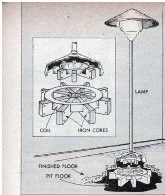
Cordless floor lamp relies upon induction coil buried in concrete slab floor, secondary coil in lamp base
